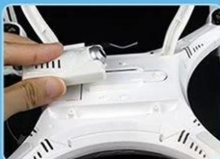
Fit the camera into the battery cover slot
