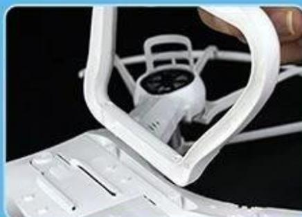
Mount the landing gear onto the bottom of the aircraft
