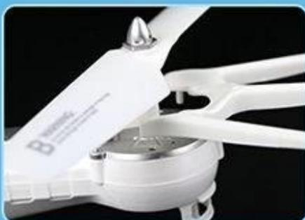
Install the protective frame onto the small holes below the blade
