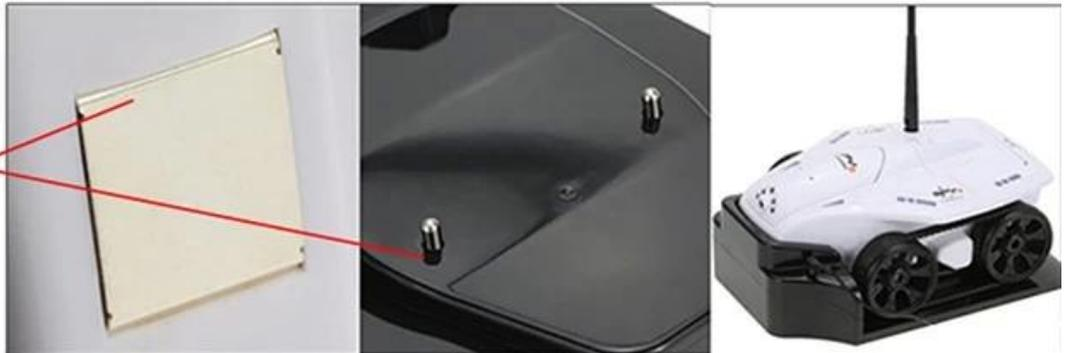
2. Put the tank on the charging seat correctly.
