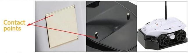
2. Put the tank on the charging seat correctly.
